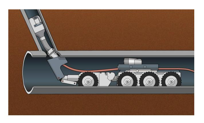
...allowing inspection of laterals from the sewer main.
