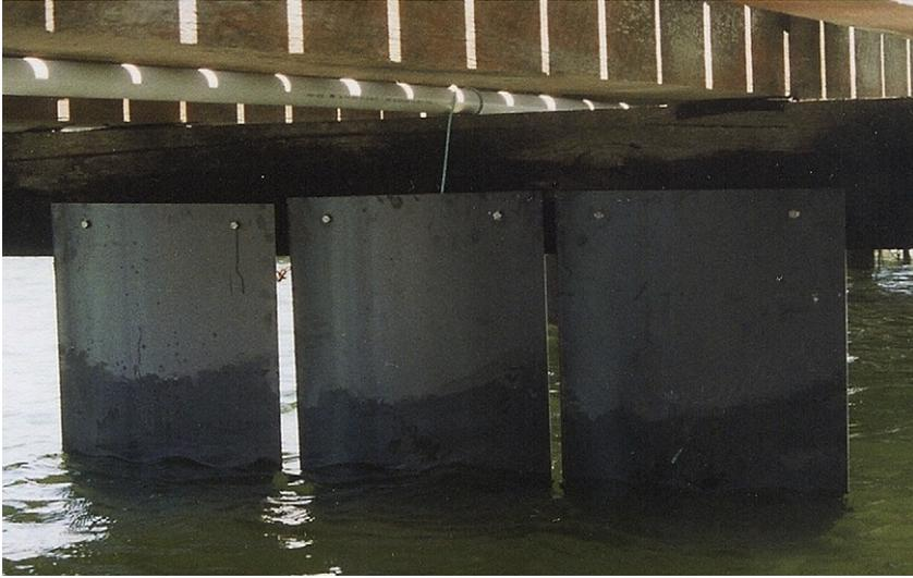
**Fig. 1.** Steel plates immediately after being suspended under jetty at Taylors Beach. [SCAN0039a.jpg.
