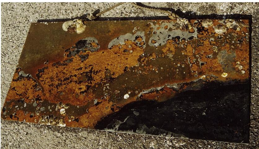
**Fig. 4.** The same plate as in Fig. 3 immediately after washing with high-pressure water. Note the appearance of some bright metal in the region of the transition zones between mud and tidal and tidal and splash zones. [SCAN0045a.
