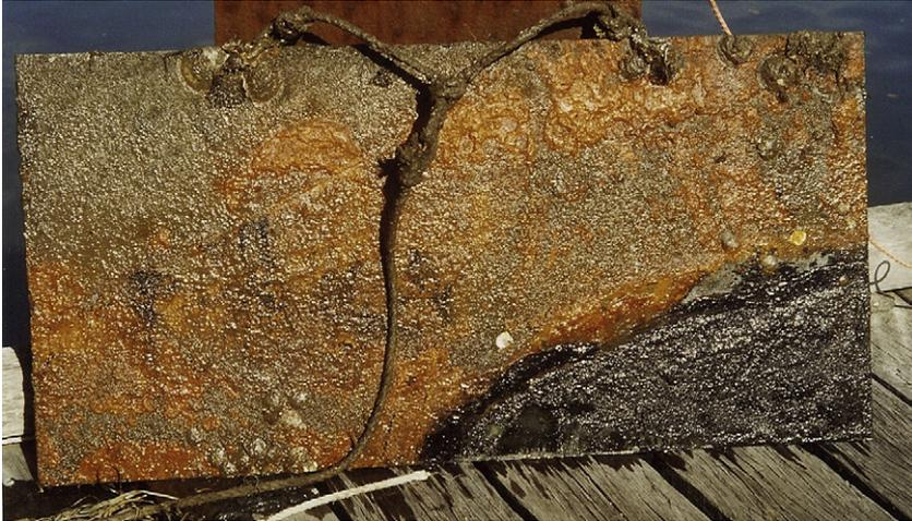
**Fig. 3.** Plate recovered from mid-estuary at 12 months exposure, showing that it inclined into the mud (at lower right). Note the distinctly different external rusts. [SCAN0044a.
