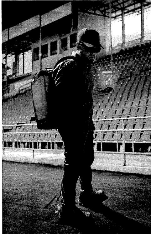
Figure 1: FlexSpec X5400 PDM deployed in its backpack configuration with smartphone user interface
