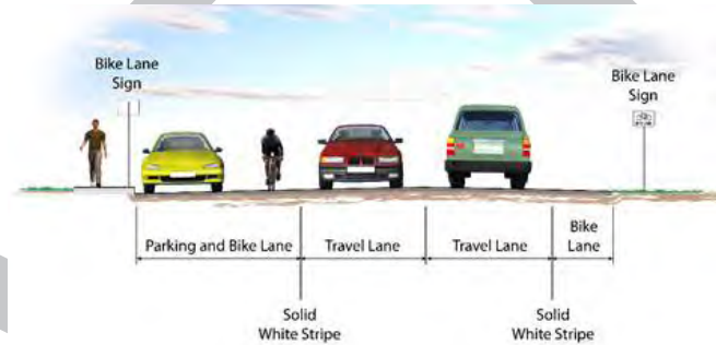
Class II- Bike Lane Provides a striped lane for one-way bike travel on a street or highway.
