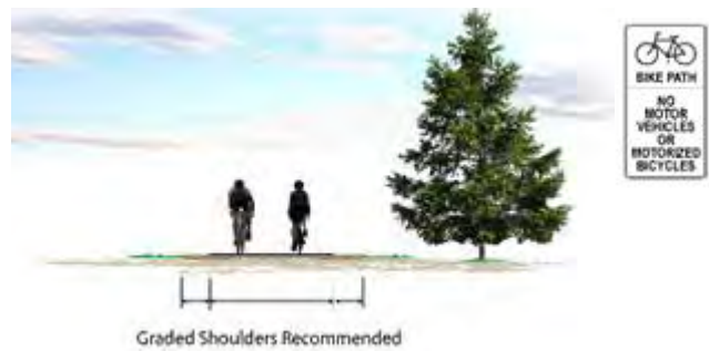
Class I- Multi-Use Path Provides a completely separated right-of-way for exclusive use of bicycles and pedestrians.
