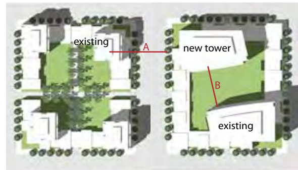
A 80-foot minimum to any existing tower across the street B 80-foot minimum to any existing tower on the same site Illustration of minimum spacing between towers.
