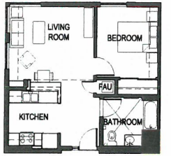
A6 - 1 BEDROOM UNIT PLAN (7) 606 SF OCCURS 1 TIME SCALE: 1/8" = 1'-0" (ON 30" X 42" SHEET SIZE)
