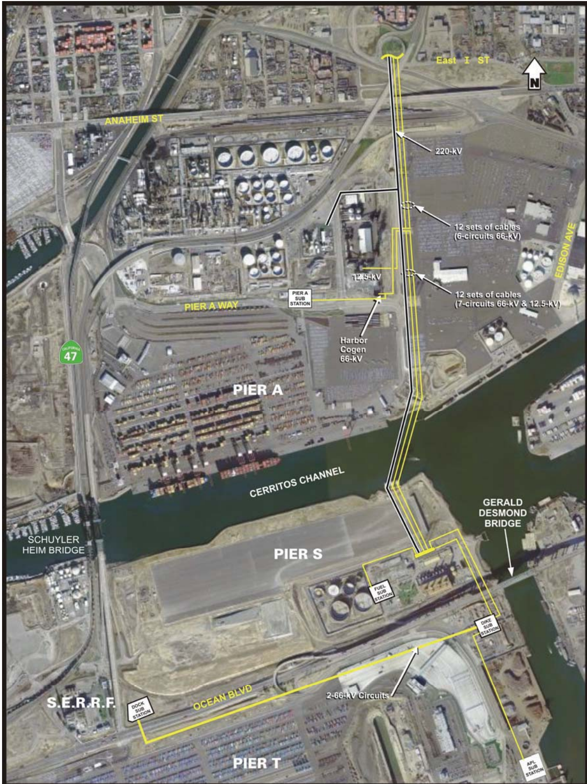
Figure 2 Existing Electrical Placement
