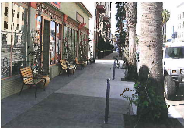
Street trees and street furnishings shall be placed outside of the primary circulation route (above). Permeable materials such as decomposed granite (below) can be used to allow additional room for pedestrian circulation.
