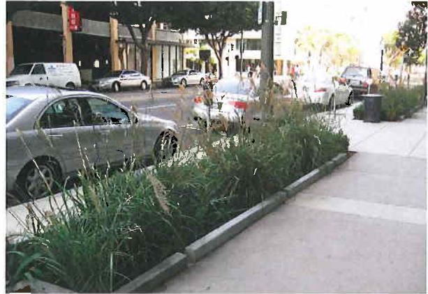
Parkway planting shall be set back 18 inches from the curb to allow for easy access to parked vehicles.
