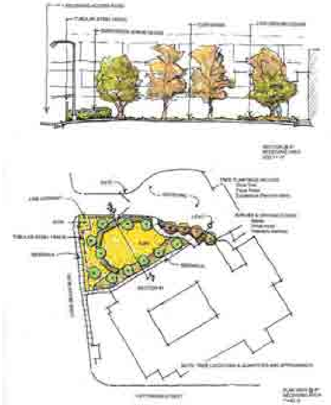
FIGURE 5.23 - Edge Treatment of Interior Sidewalks
