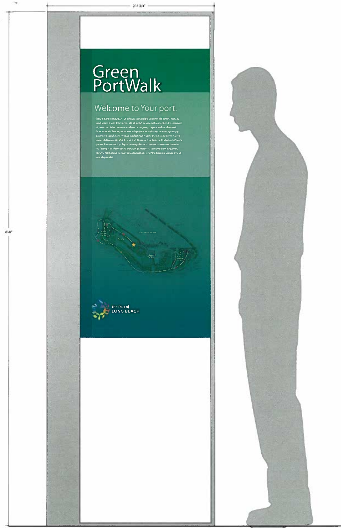
X04 TRAIL ENTRY MARKER Elevation - Front View SCALE: 3/4" = 1'-0"
