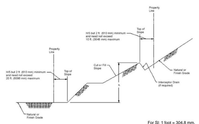
FIGURE 18.75.060 DRAINAGE DIMENSIONS
