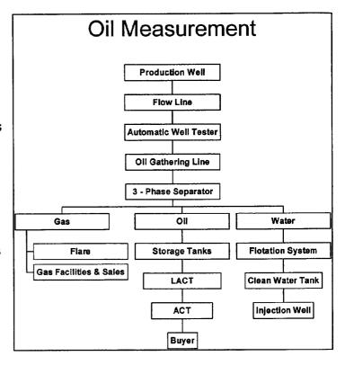
There are two ACT units located near the intersection of Broadway and Pico Avenues (aka Broadway-Mitchell site) that alternatively measure the amount of oil shipped. These ACT units are connected to five separate buyer's pipelines, including, ARCO (two lines), Mobil, Conoco/Phillips, and Equilon. Run tickets are used to document the transfer of ownership of oil.
