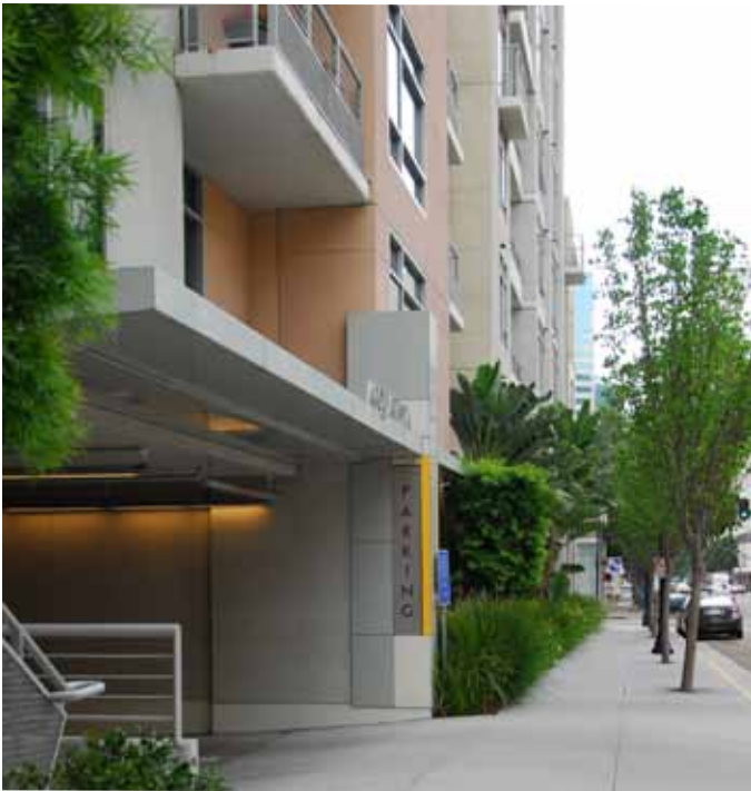
Garage entrances should be incorporated into the building's architecture, be well signed and, where possible, should complement other ground-floor uses (above).
