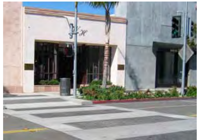
Where possible, crosswalk paving shall visually tie into the adjacent streetscape and contrast with the adjacent street paving.
