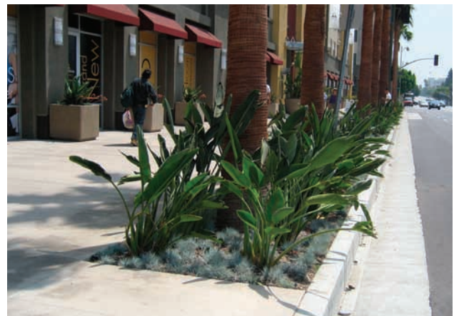
Parkway planting should be used to buffer the street from the pedestrian zone and minimize paving where curb-to-building sidewalks are not needed, such as along residential streets.
