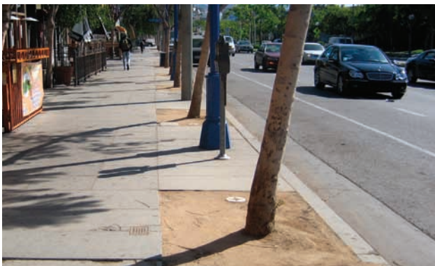
Street trees and street furnishings shall be placed outside of the primary circulation route (above). Permeable materials such as decomposed granite (below) can be used to allow additional room for pedestrian circulation.
