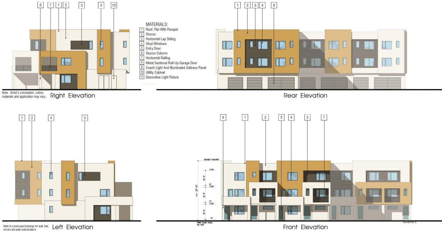
Figure 8 Project Elevations – Building 700 Townhome Elevations
