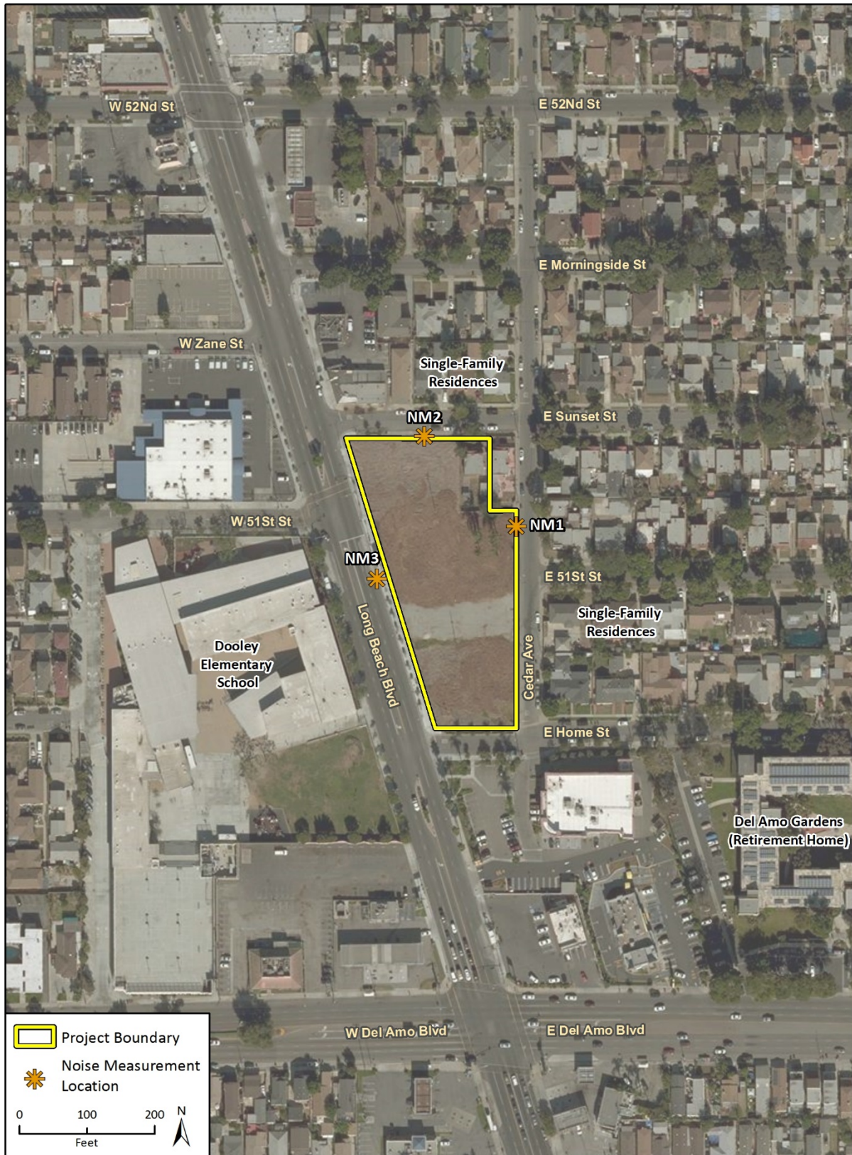
Figure 10 Sound Level Measurement and Sensitive Receptor Locations
