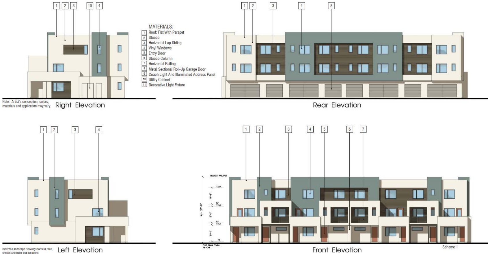
Figure 9 Project Elevations – Building 800 Townhome Elevations
