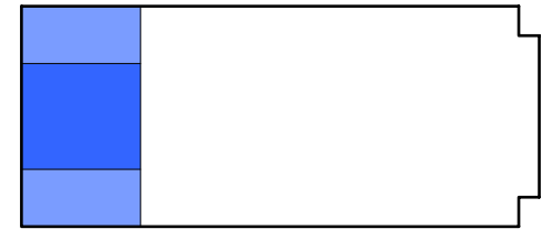
PRACTICE SYNCHRONIZED SWIMMING 25 YD x 12 M x 2 M DEEP W/ 12 M x 12 M x 3 M DEEP SECTION WITHIN
