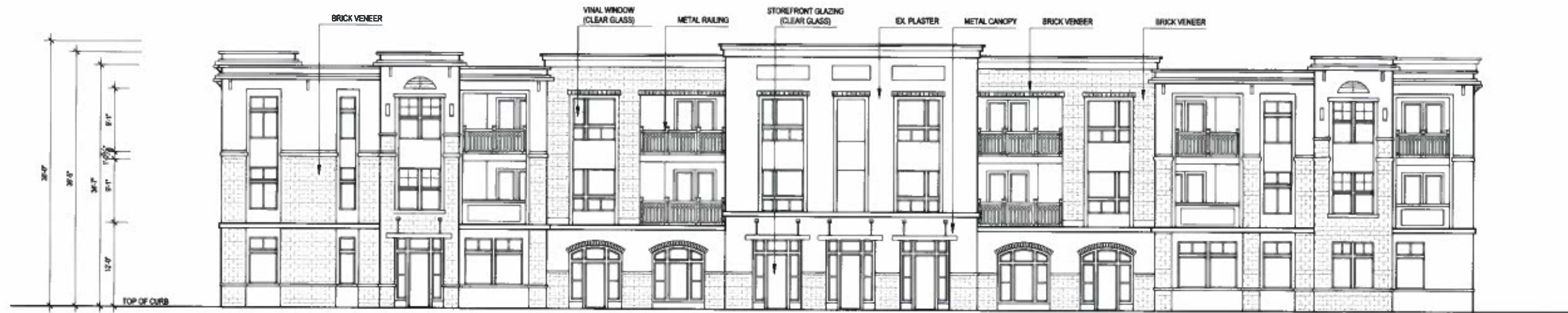
NORTH ELEVATION (ALONG EAST ARTESIA BLVD.) SCALE: 1/8" = 1'-0"
