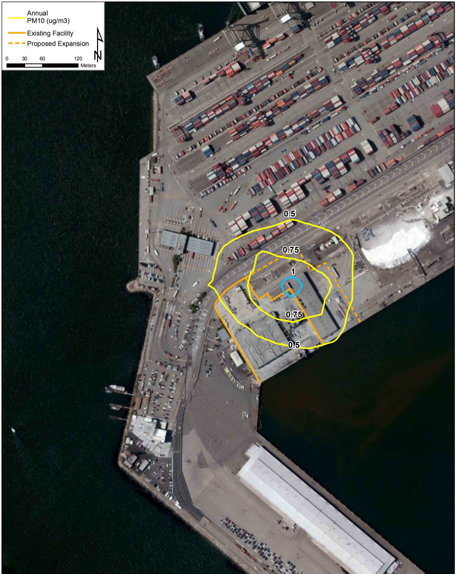
Figure A-2-13. Maximum Annual PM10 No Project minus CEQA Baseline Impacts (ug/m3)
