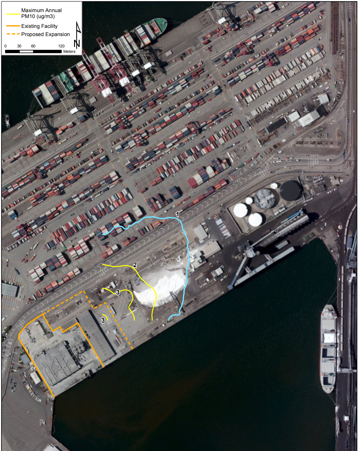
Figure A-2-8. Maximum Annual PM10 Mitigated Project minus CEQA Baseline Impacts (ug/m3)
