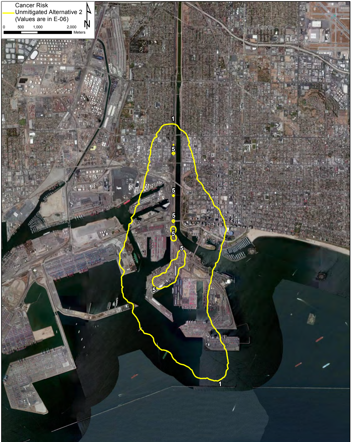
Figure A-3-5. Unmitigated Alternative 2 Cancer Risk Isopleths (probability per million of causing cancer).
