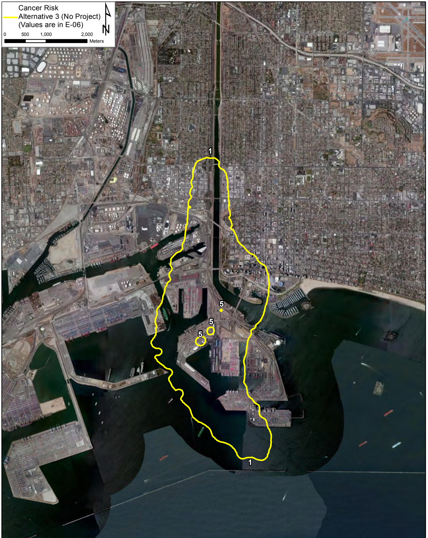
Figure A-3-7. Unmitigated Alternative 3 (No Project) Cancer Risk Isopleths (probability per million of causing cancer).
