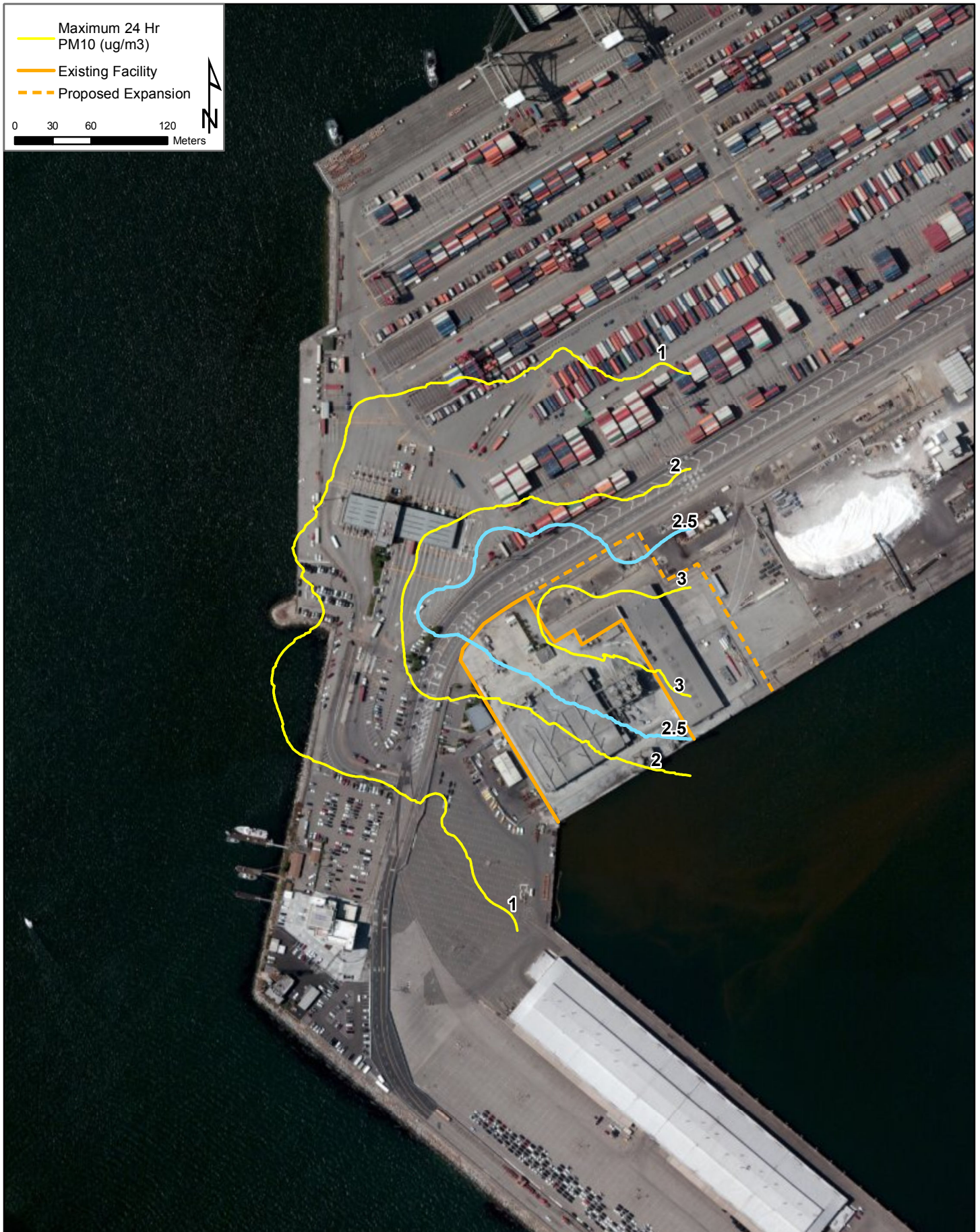
Figure A-2-12. Maximum 24-Hour PM10 No Project minus CEQA Baseline Impacts (ug/m3)
