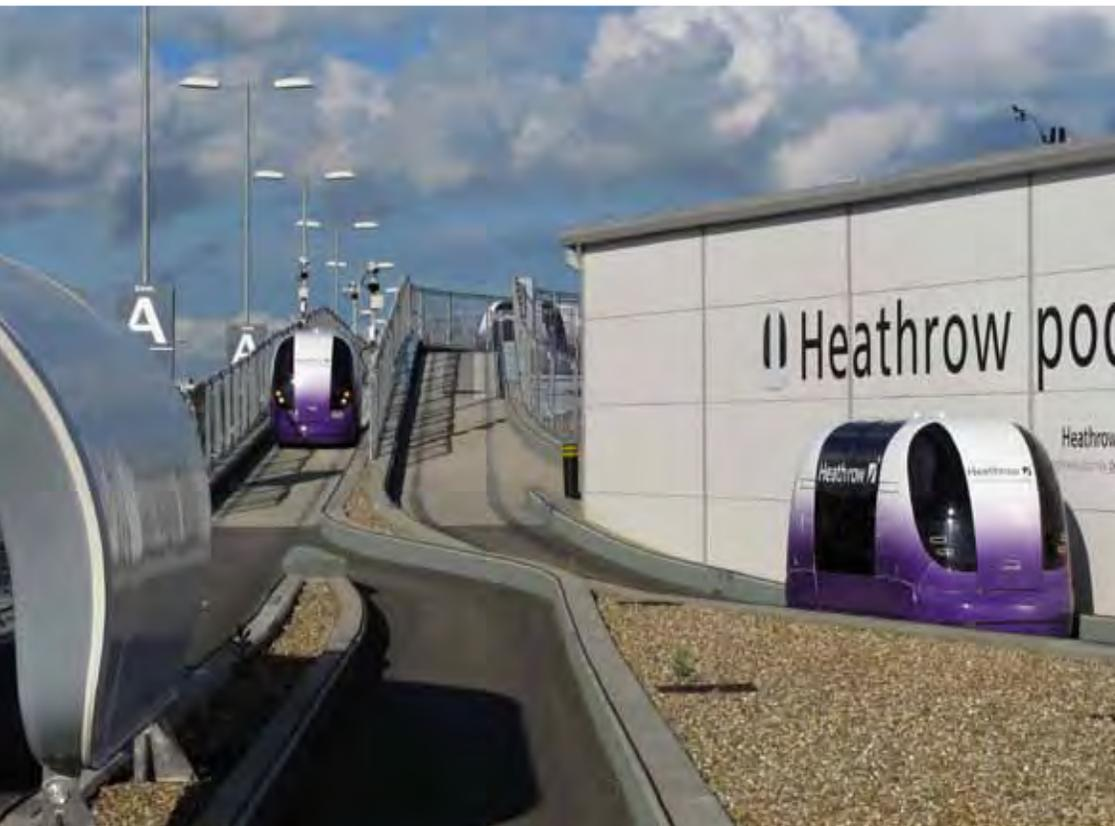
*London's Heathrow Airport pod is an on-demand and nonstop personal rapid transit that carries passengers traveling between the terminals and parking garages. The personal rapid transit addresses the need to move commuters in areas where the densities were too low to pay for the construction of a conventional light rail.*
