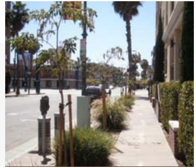
Figure 2.54 Permeable boulevard plantings along 4th Street helps reduce polluted runoff and recharge groundwater.
