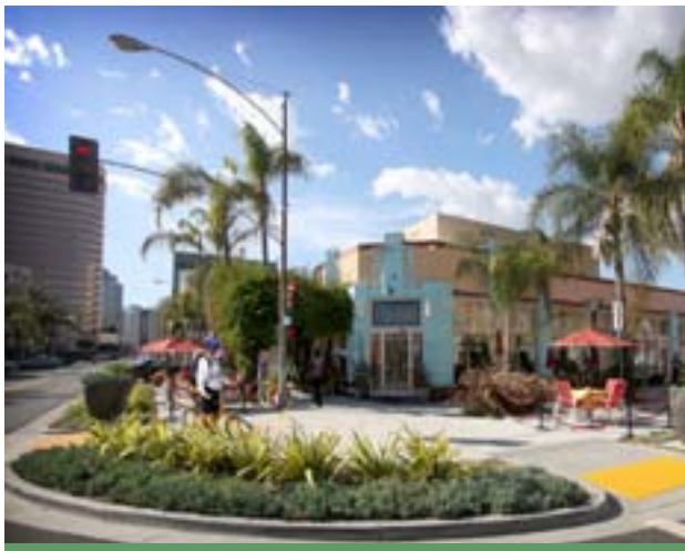
Image 4.1 Curb Extension - 1st Street and Linden Avenue, Long Beach, CA.
