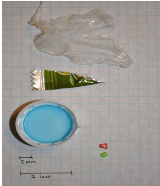
Figure 6-5 Sample reference photographs can help identify the sizes of debris based on visual cues like grids. The red pellet is about 5 mm long. Photo: Michael Mori
