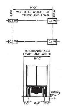
Note: The H loadings consist of a two-axle truck or the corresponding lane loadings as illustrated above. The H loadings are designated "H" followed by a number indicating the gross weight in tons of the standard truck.
