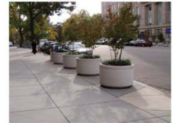
Precast concrete planter pots with anti graffiti coating treatment. Planted with drought tolerance plants.
