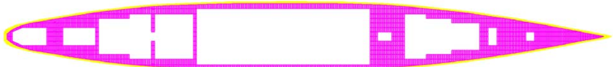
C Deck (elevation 46'-6", plating 0.38")
