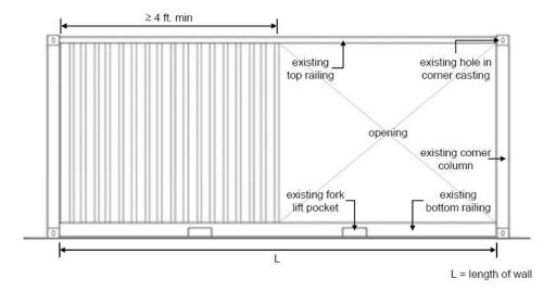
FIGURE 3114.8.5.3(2) Bracing Unit Distribution – Minimum Linear Length
