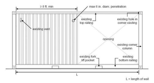
FIGURE 3114.8.5.3(4) Bracing Unit Distribution – Penetrating Limitations
