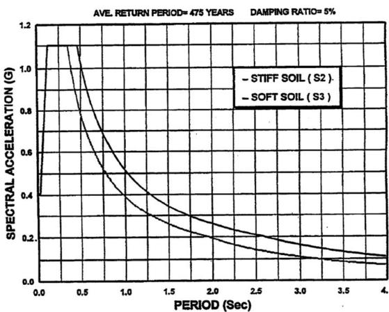
FIGURE 71-1 RESPONSE SPECTRA SHAPES
