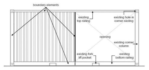
FIGURE 3114.8.5.3(3) Bracing Unit Distribution – Boundary Elements
