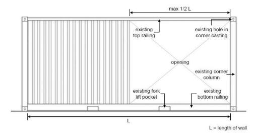
FIGURE 3114.8.5.3(1) Bracing Unit Distribution – Maximum Linear Length
