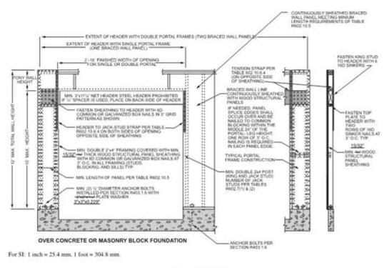
FIGURE R602.10.6.4 METHOD CS-PF—CONTINUOUSLY SHEATHED PORTAL FRAME PANEL CONSTRUCTION
