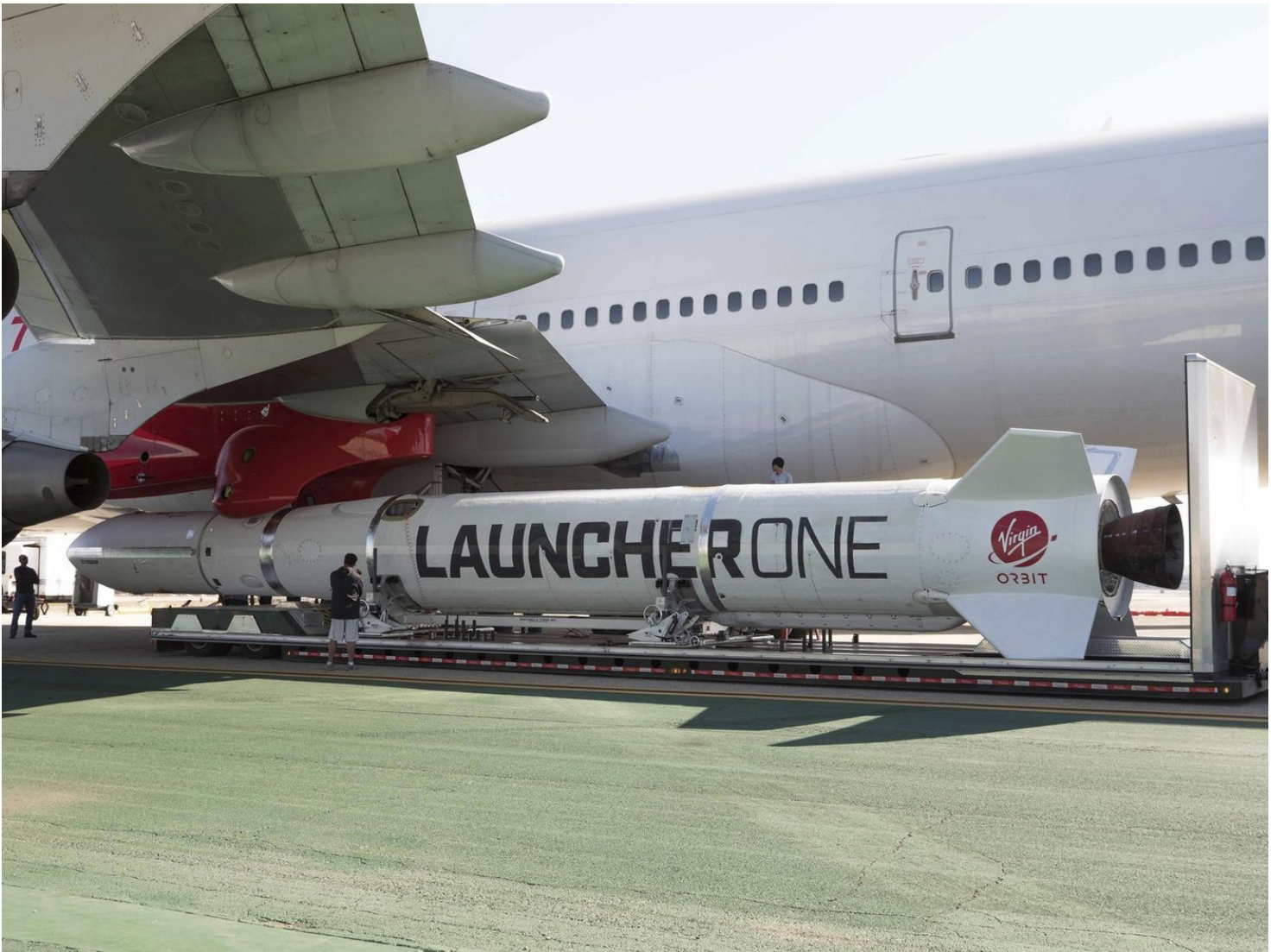
In this Thursday, Oct. 25, 2018, photo released by Virgin Orbit, a completed LauncherOne rocket hangs from the wing of Cosmic Girl, a special Boeing 747 aircraft that is used as the rocket's "flying launch pad," at the Long Beach Airport in Long Beach, Calif. The system is intended to carry small satellites into orbit. Virgin Orbit is a sister company of Virgin Galactic, which is developing an air-launched rocket plane for carrying tourists on suborbital flights into space. (Greg Robinson/Virgin Orbit via AP) (AP)
