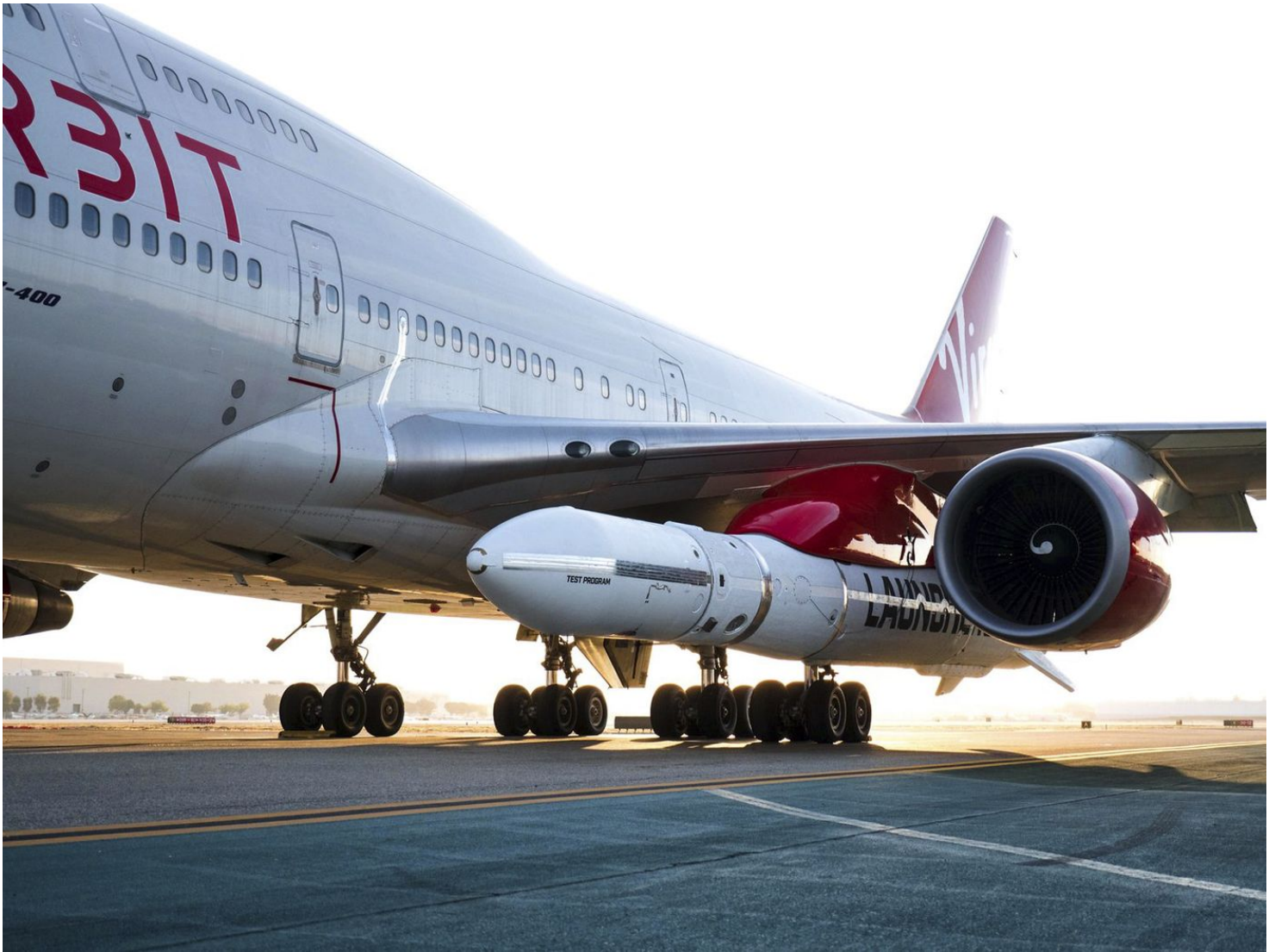
In this Thursday, Oct. 25, 2018, photo released by Virgin Orbit, a completed LauncherOne rocket hangs from the wing of "Cosmic Girl," a Boeing 747 aircraft used as the rocket's "flying launch pad," at the Long Beach Airport in Long Beach, Calif. Southern California-based Virgin Orbit has reached a milestone in developing its airborne orbital launch system. Virgin Orbit is a sister company of Virgin Galactic, which is developing an air-launched rocket plane for carrying tourists on suborbital flights into space. (Greg Robinson/Virgin Orbit via AP) (AP)
