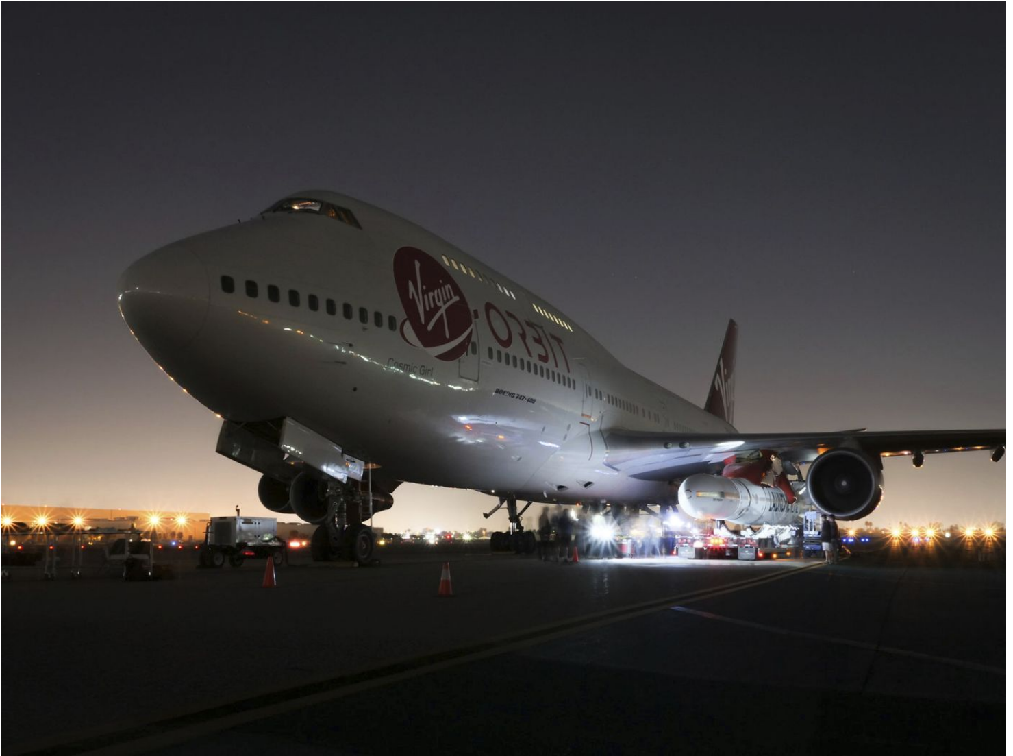
In this Wednesday, Oct. 24, 2018, photo released by Virgin Orbit, a completed LauncherOne rocket hangs from the wing of Cosmic Girl, a special Boeing 747 aircraft that is used as the rocket's "flying launch pad," at the Long Beach Airport in Long Beach, Calif. The system is intended to carry small satellites into orbit. Virgin Orbit is a sister company of Virgin Galactic, which is developing an air-launched rocket plane for carrying tourists on suborbital flights into space. (Greg Robinson/Virgin Orbit via AP) (AP)
