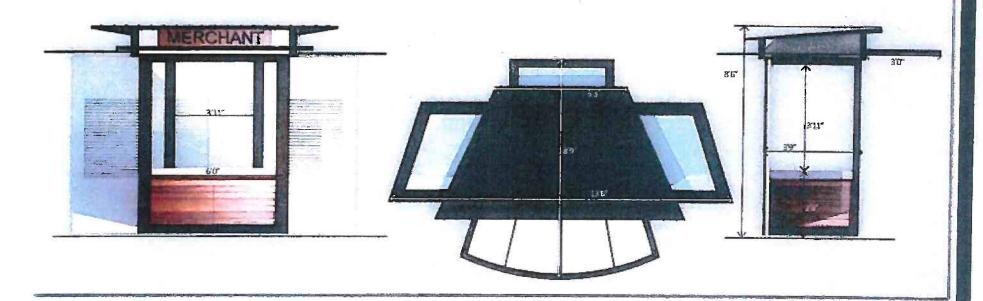
Locking Security Doors Pull-Out Shelf w/Lip Cashwrap w/Pull-Out Shelf Locking Door w/Storage Metal Awning UV Protected Awning Panel [Optional] Teak Wood Plank Columns w/Roll Down Tracks Door Stop w/Sealing Gasket [9] Recessed Lights Tenant Signage Solid Surface Countertop
