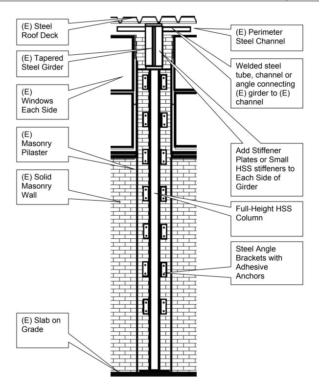
Interior Elevation of Schematic Pilaster Strengthening at Assembly
