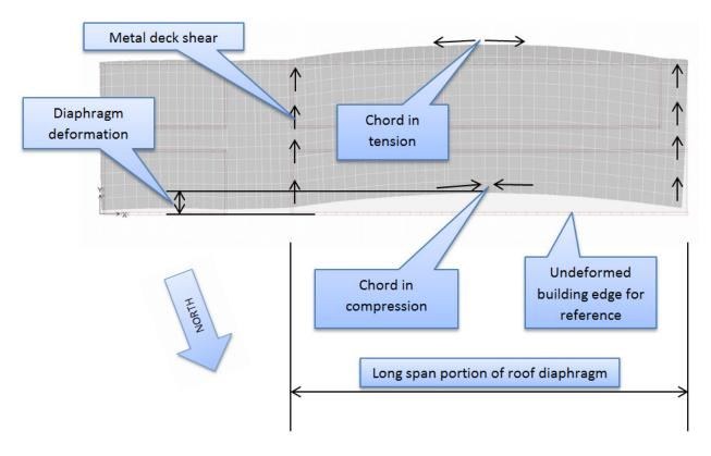
Main Wing Partial Roof Plan Showing Diaphragm Behavior
