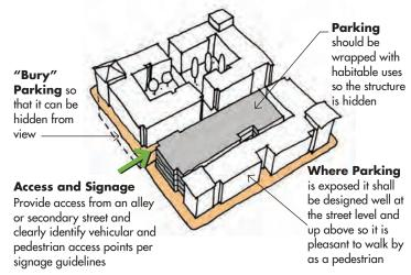
Ideally, garages should be hidden from view or located underground or behind habitable uses as shown here. The exception occurs when a garage provides an active ground-floor use or can prove its contribution to Downtown with an outstanding architectural presence on the street.
