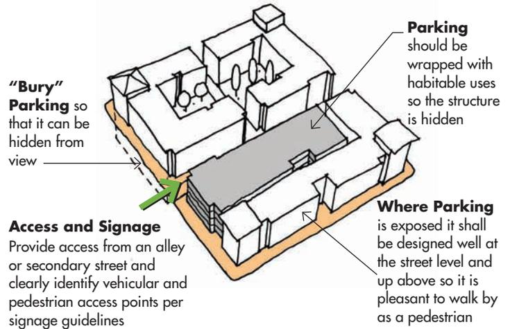
Ideally, garages should be hidden from view or located underground or behind habitable uses as shown here. The exception occurs when a garage provides an active ground-floor use or can prove its contribution to Downtown with an outstanding architectural presence on the street.
