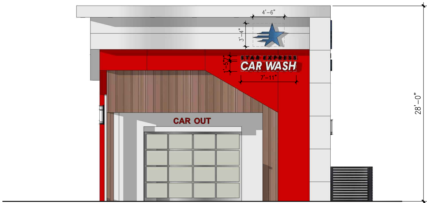
SOUTH ELEVATION - WASH BLDG. SCALE: 1/8" = 1'-0"
