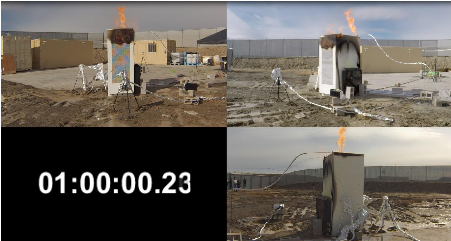
Figure 22 External test screenshot: test time = 1 hour, fire emanating from the front door and exhaust vent, pops consistent with battery cell thermal runaway heard steadily, burners turned "OFF"
