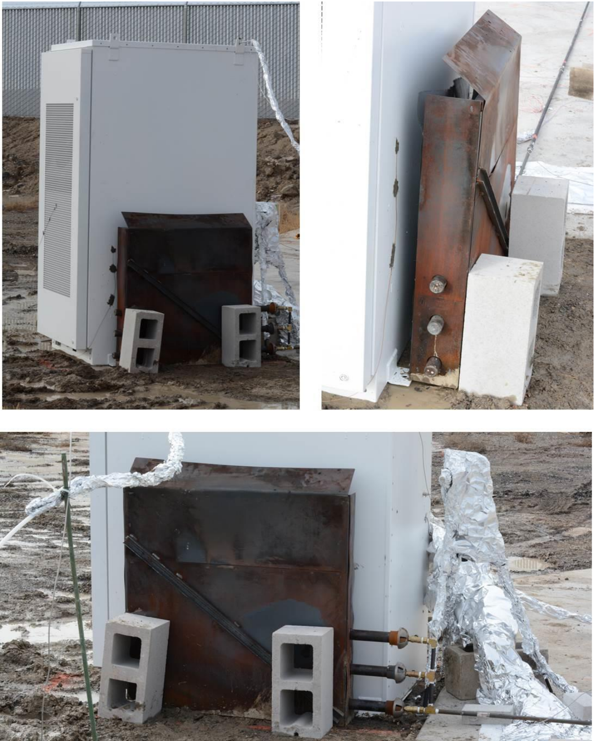
Figure 13 Burner assembly and positioning
