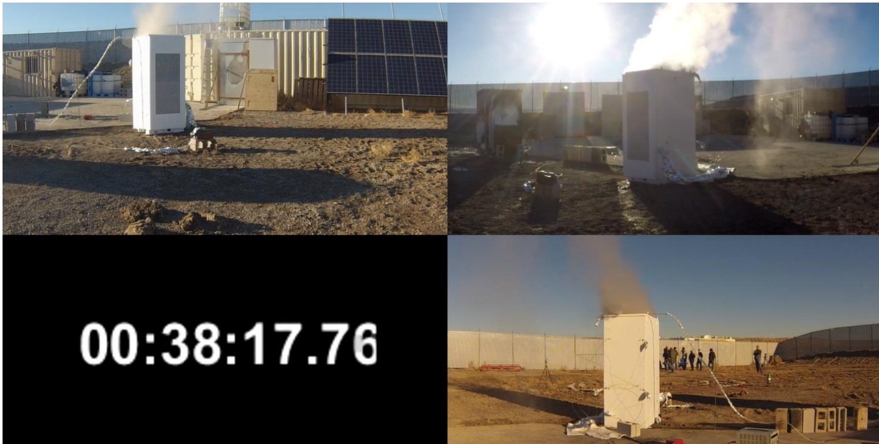
Figure 30 Internal test screenshot: peak smoke production approximately 35 to 40 minutes after the heater cartridges were turned "ON"
