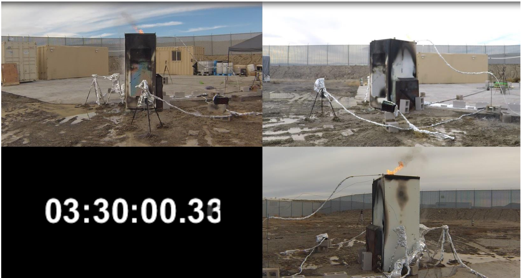
Figure 27 External test screenshot: test time = 3 hours 30 minutes, fire inside the Powerpack burning itself out
