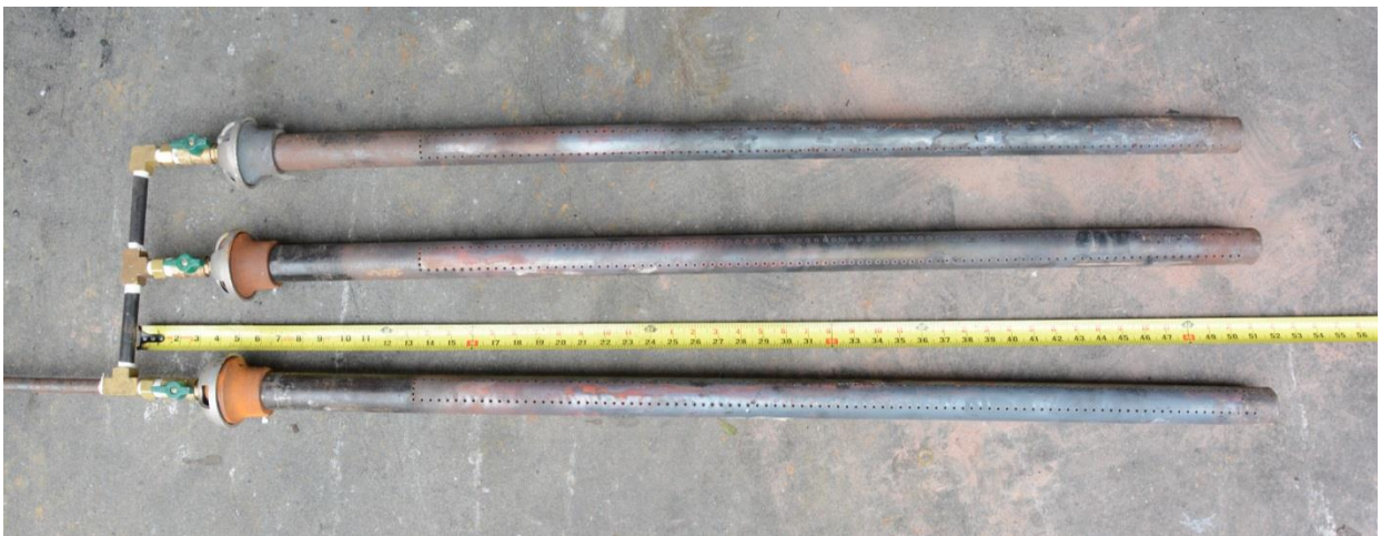
Figure 12 Burners utilized for testing
