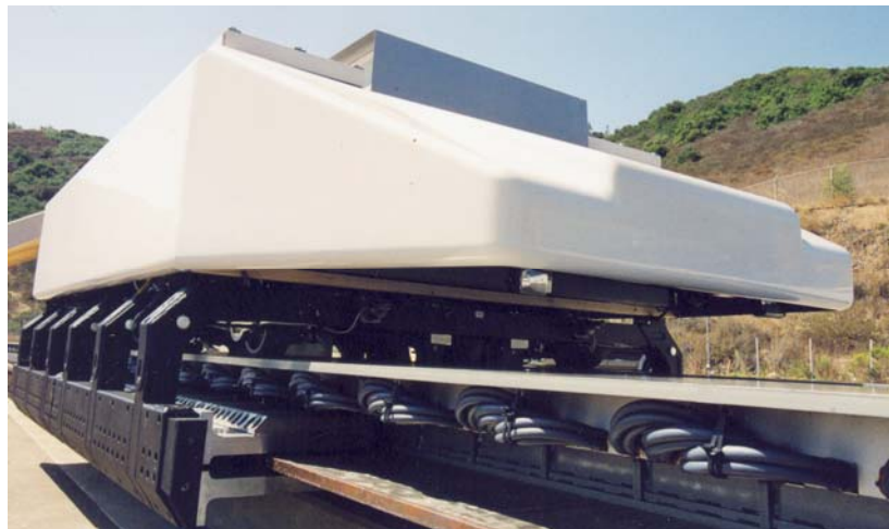
Fig. 3-11. ECCO levitated on guideway (top figure); test chassis unit on the test track at GA (lower figure); each ECCO has seven chassis units
