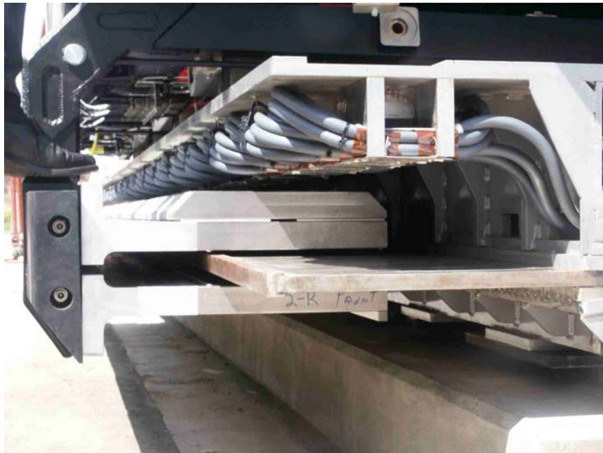
Fig. 3-5. Existing levitation propulsion arrangement of the urban maglev chassis
