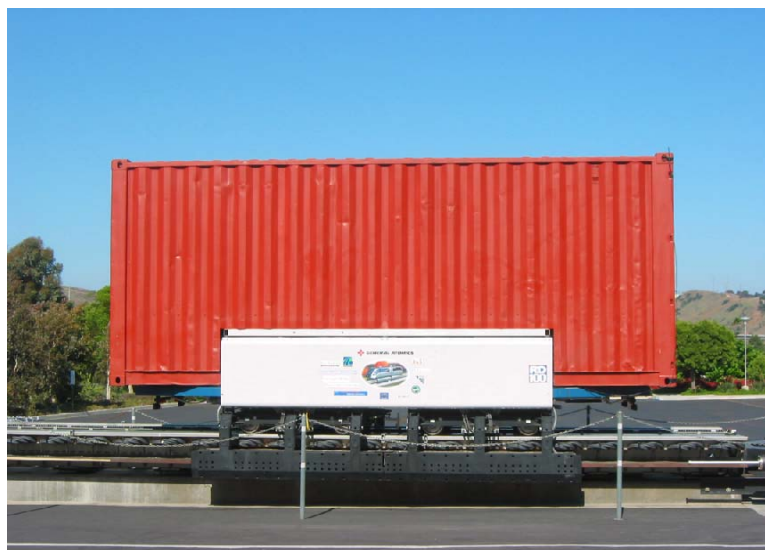
World’s first cargo maglev system, the Electric Cargo Conveyor (ECCO) undergoes testing at the GA test track in San Diego, California
