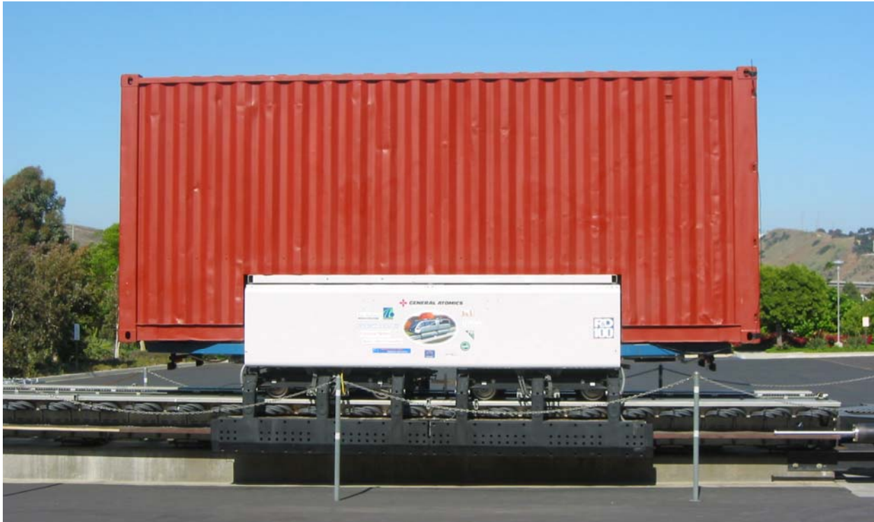
Fig. 1-2. GA maglev vehicle testing at the test track in San Diego, California
