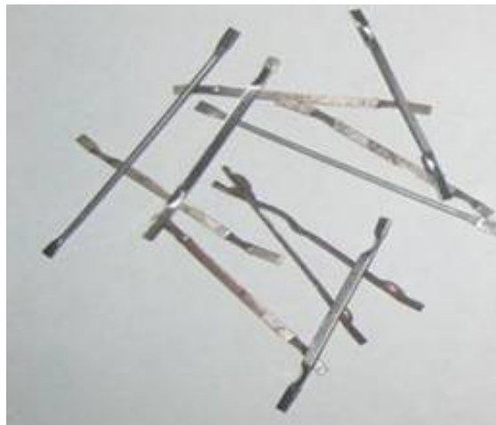
Fig. 3-21. Fibers in the SFRC concrete
