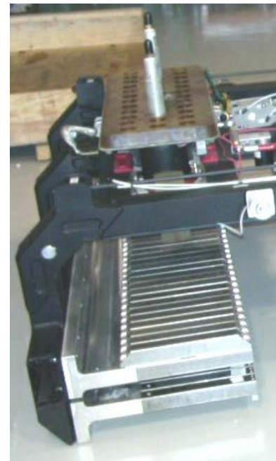
Magnets used for levitation and propulsion are robust, off-the-shelf components
