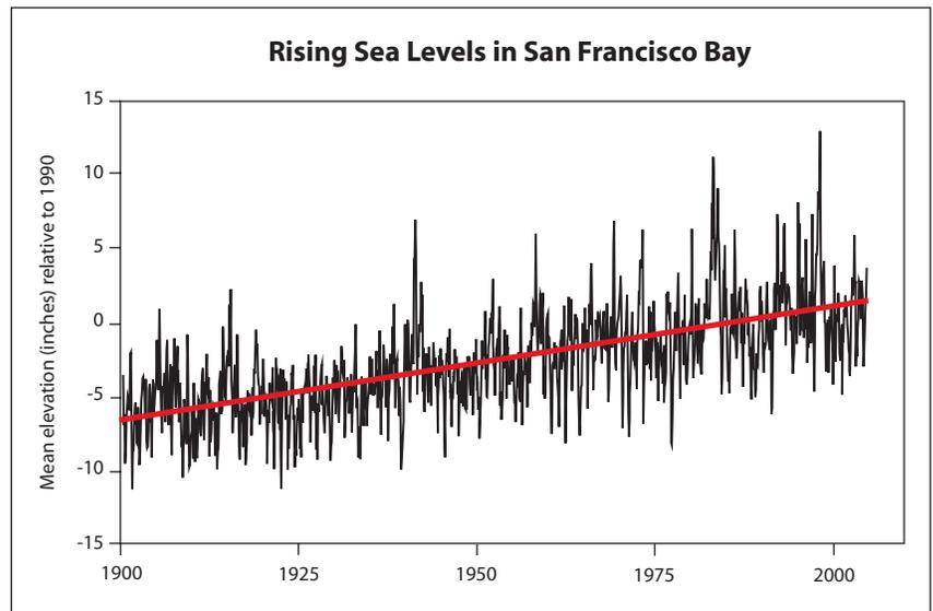
Although levees have been built to contain the 100-year flood, a 12-inch increase in sea levels (projected for the medium warming range of temperatures) would mean storm-surge-induced flood events at the 100-year level would likely occur once every 10 years.
