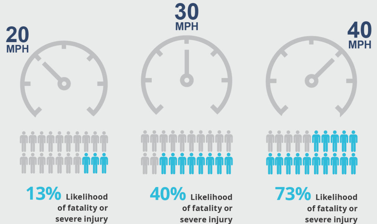
Figure 4. How Speed Kills - Relationship between Motor Vehicle Speed to Pedestrian Fatalities and Serious Injuries
