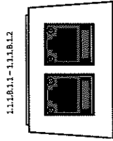
DETAIL #4 2-PORT SURFACE MOUNT WAP (2-C6A)
