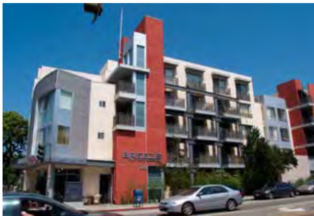
Horizontal variation can be provided with changes in the streetwall plane, materials, and color.
