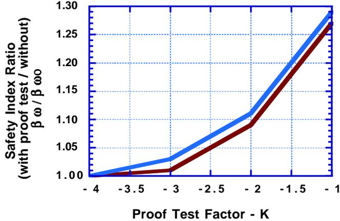
Fig. 6: Effects of proof testing on pipeline reliability
