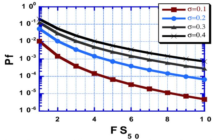
Fig. 2: Probability of failure as function of central Factor of Safety and total uncertainty
