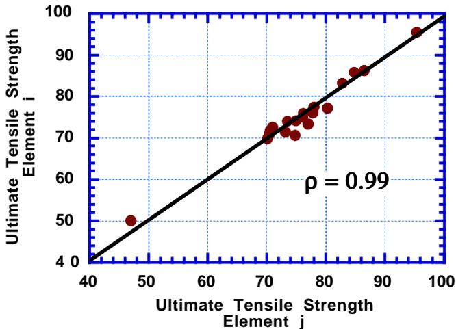
Fig. 14: Correlation of measured ultimate tensile strengths of paired pipeline steel samples from adjacent pipeline segments
