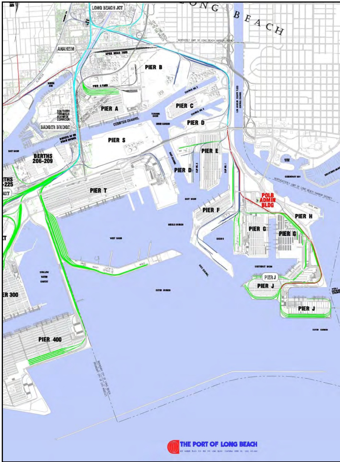
Figure 3-2: Port Vicinity Rail Facilities
