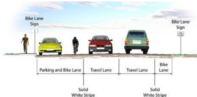
Class II – Bike Lane Provides a striped lane for one-way bike travel on a street or highway.
