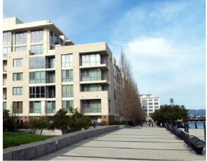
Setbacks make building heights less imposing and create variation in building massing.
