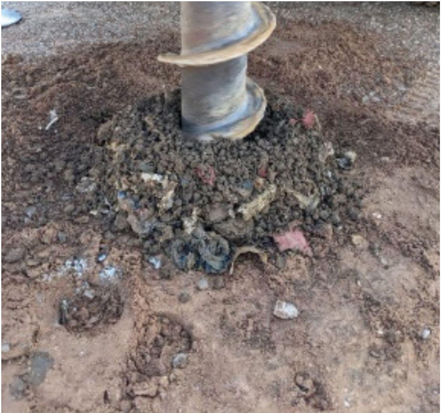
Photo 2: Drill cuttings consisting of landfill material from the subsurface
