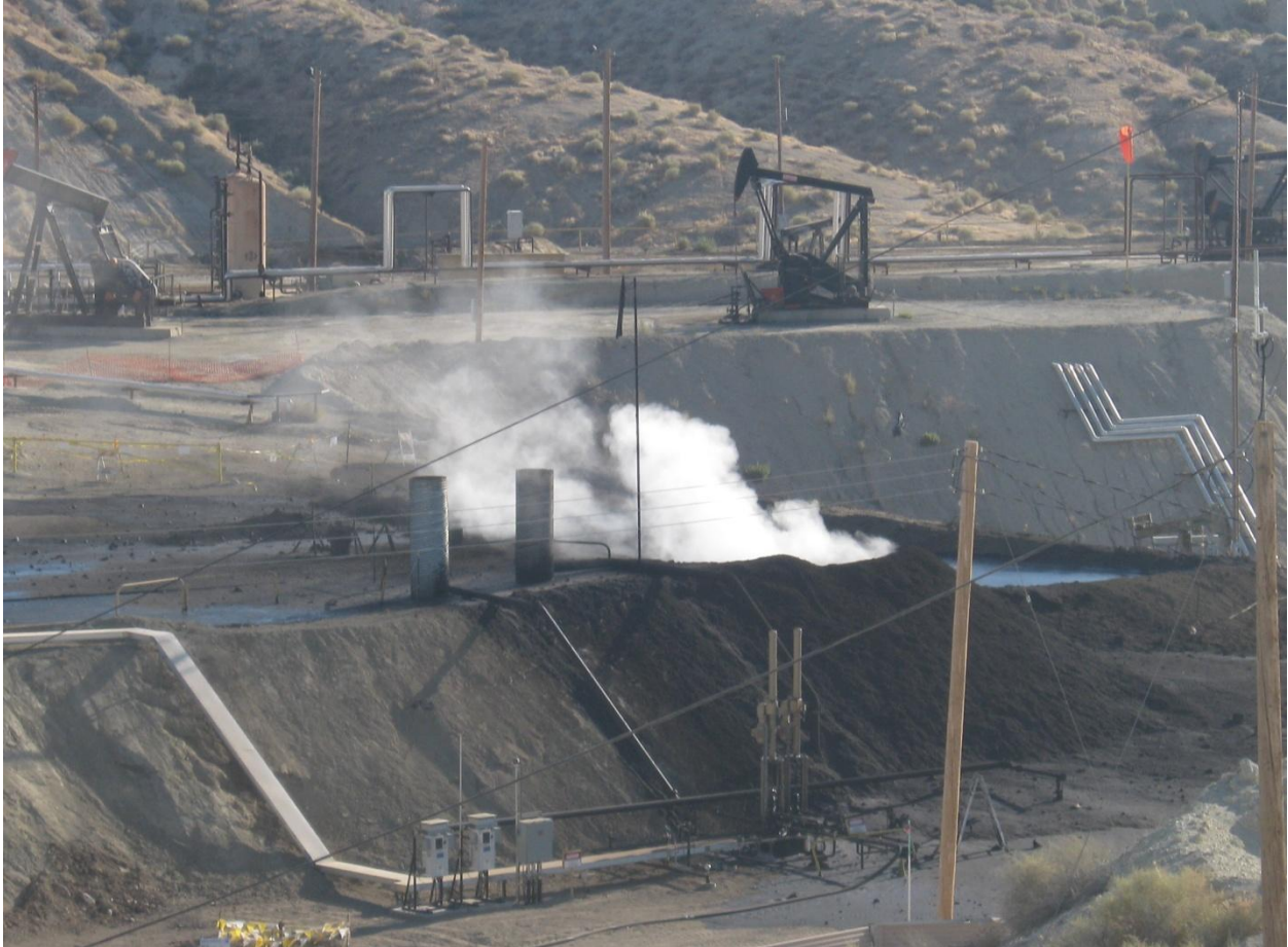
Photograph 24 – View of Chevron Well 20 surface expression crater on August 18, 2011 one day after the large August 17 eruption. Plumes of steam continued to rise from crater for several days following the event.
