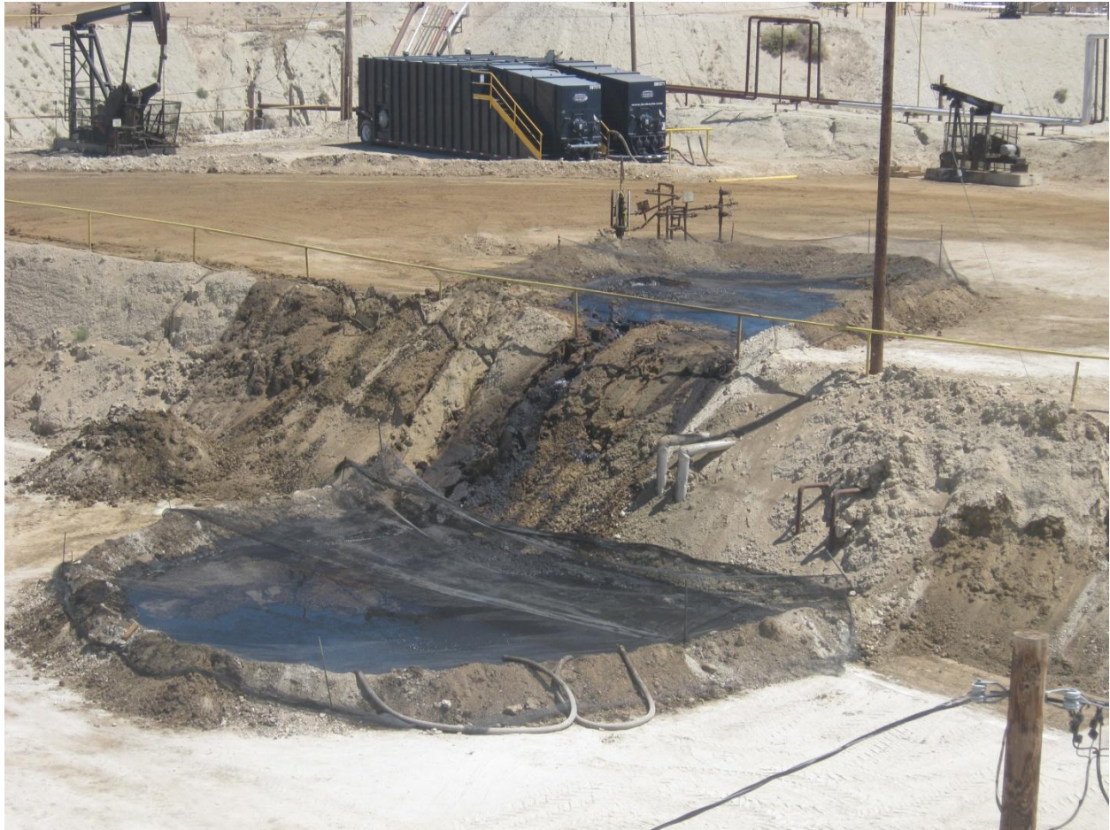
Photograph No. 12 - View of the June 22, 2011 surface expression on TRC Operating Company's "Bull" lease, section 22 T32S/R23E. Crater of the surface expression can be seen on the upper terrace above yellow horizontal guard post. Approximately 600 bbls of fluid were reportedly removed from the bermed pit in 48 hours and approximately 1000 bbls of fluid over the first week of activity. This location is approximately 400 feet from the Chevron accident site.
