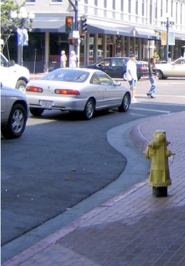
Bulbouts could provide an enhanced pedestrian experience in the SEASP area by shortening the distance it takes to cross the street.
