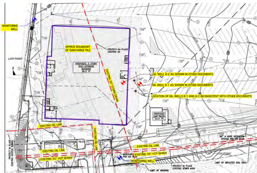
Figure 3. Diagram of Premature Surcharge Program.
