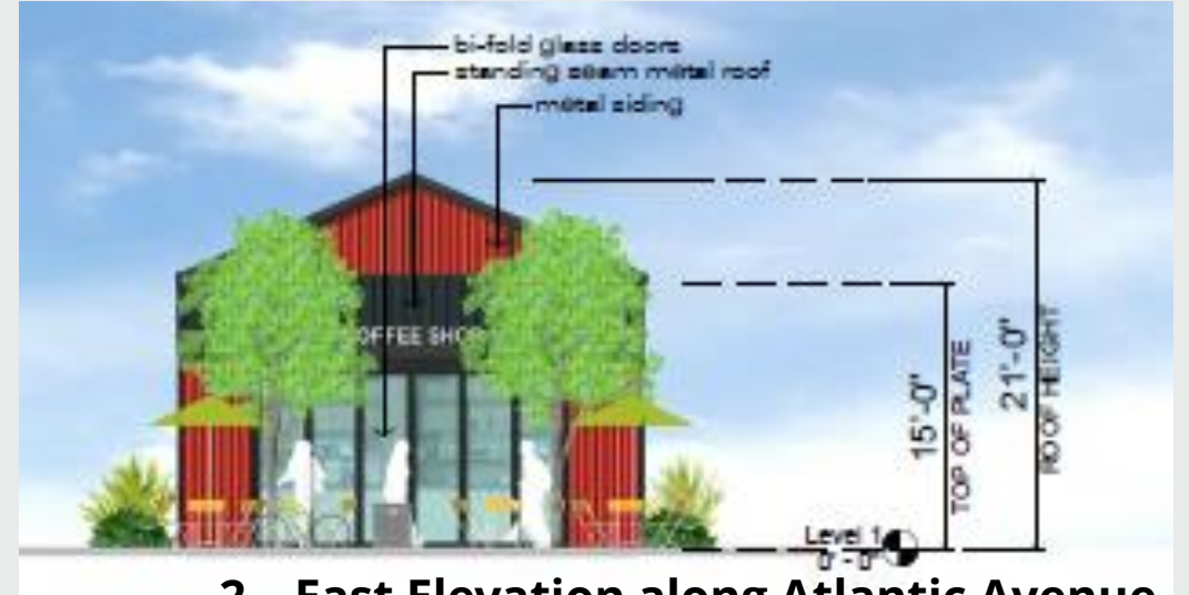
2 – East Elevation along Atlantic Avenue
