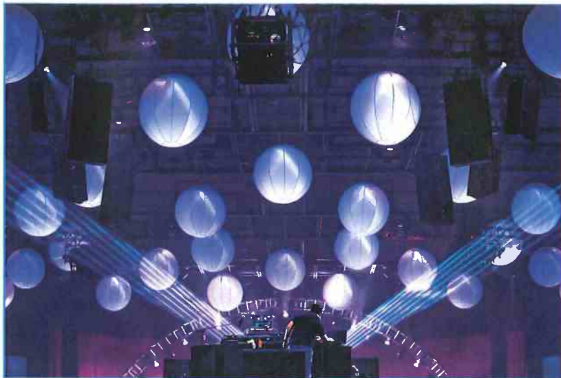
Renkus-Heinz IC 2 cabinets require no articulation between enclosures since steering/aiming is accomplished via computer-controlled DSP.
