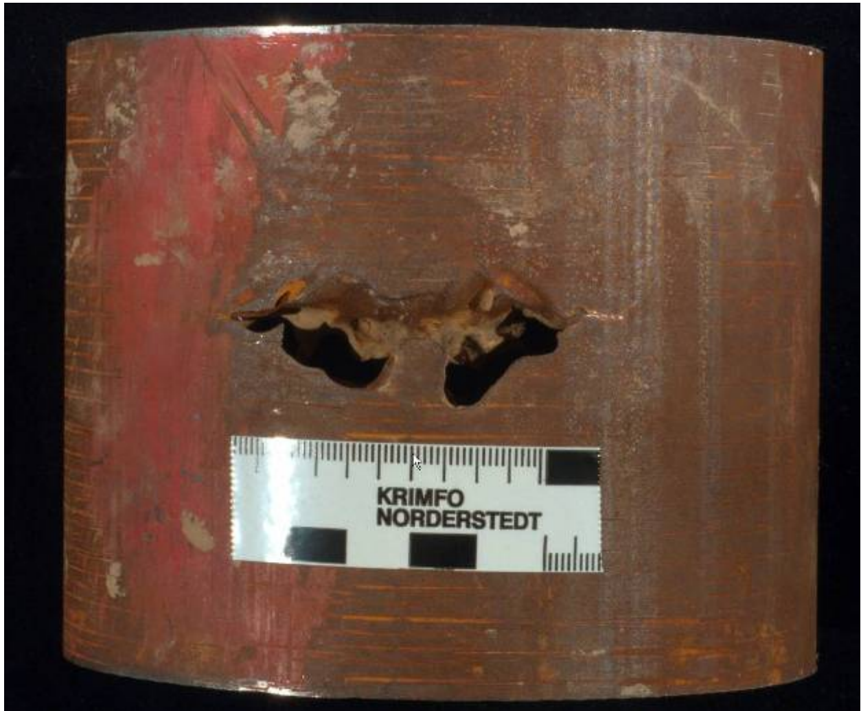
Figure 6-2 Typical example wash-out of drill string (DNV photo).
