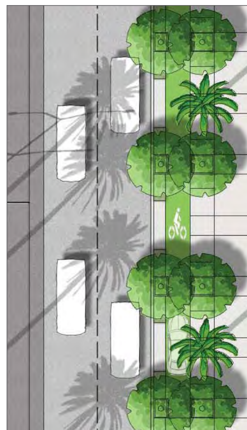
A class IV bike lane, also known as a cycletrack (protected bike lane), could be considered for Long Beach Boulevard if on-street parking is no longer needed.
