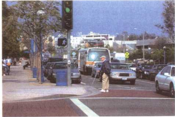
Sidewalk extensions at crosswalks make it easier for pedestrians to cross the street.
