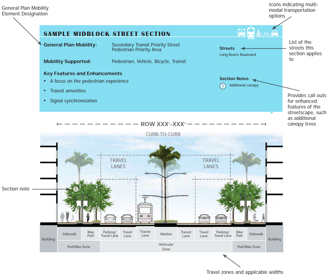
FIGURE 4-4 GUIDE TO TYPICAL MIDBLOCK STREET SECTIONS
